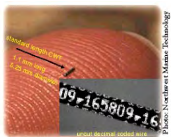
Above: Standard length coded wired tag.
